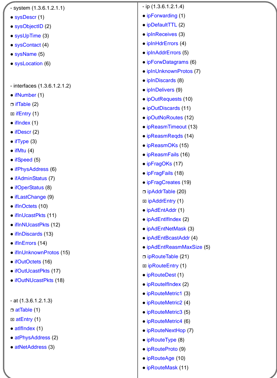
Figure 2-2 Tree Structure for MIB-II System, Interfaces, AT, and IP Groups
